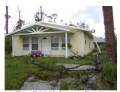
This affordable home in Florida withstood the damage of Hurricane Charley in 2004. It was built with fibercement-faced structural insulated wall panels and survived 145 mph winds. The insulated panels are also highly energy efficient.
