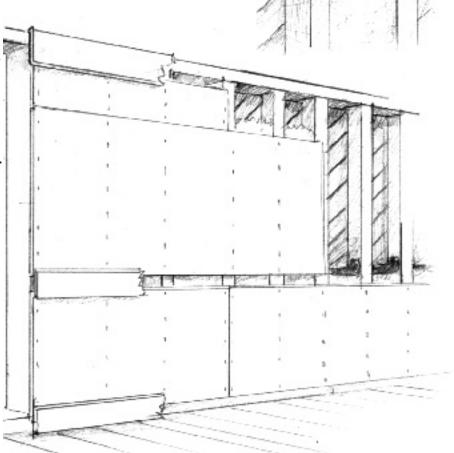
Where the roof has soffit vents, install collar ties. Install gable end vents above the collar ties at both ends. Install continuous sheets of 2 inch Thermax (or equivalent) under rafters and collar ties. If there is a roof vent, the gable end vents are not necessary.
