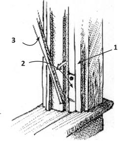
6 Pass chain over pulley (don't cut to length yet). Reach into weight compartment and pull out chain. Thread chain through eye of weight and wire chain to chain. (Use fixture if it comes with chain.) Put chain through closed loop, then weight eye, next attach chain to open hook, fixture if it comes with chain.) Put chain through closed loop,
