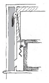
**7** Place bottom sash on window stool. Pull chain until weight contacts pulley. Let pulley down a couple of inches. Push nail through chain at pulley to hold in place. Cut off chain just below round hole in sash edge. Turn chain halfway on spring-like fixture that comes with chain.
