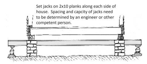
Run I-beam under sill beam (or joists if sill beam is to be removed)
