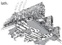
**3** Where the plaster keys are broken and plaster is pulling away from the lath, tighten loose plaster back to the lath with plaster washers. Where possible squeeze construction mastic through holes between plaster base-coat and lath. To hold assembly while drying wedge a 2x4 between the floor and a square of plywood held against the ceiling.
