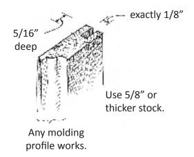
Install a nylon brush seal into the kerf and a rubber gasket between the stop and the window jamb to seal. Both can be ordered from RCT or other suppliers. Drill oval holes through stop and screw through a finish washer into the jamb. This design allows you to loosen the screw and adjust the amount of pressure the brush is exerting against the face of the sash.
