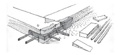
4 Clamp sash to plywood bench top (see p.75) and prepare scraps of wood that roughly fit gaps where wood has rotted away.
