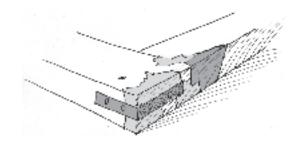
8 Perform final sanding on corner. Fill any remaining gaps as necessary.
