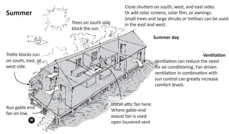
A ventilation system can range from a large window fan to a gable-end whole house fan. In either case, the fan would exhaust out from one opening other than a bedroom window. All other windows in the house, except for bedroom windows across from beds, would be kept closed at night so that cooler air is drawn across the bed. Partially closing this window will increase the velocity of air drawn from the outside.
