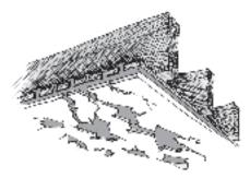
Plaster keys broken off. Keys are formed where plaster squeezes between lath and forms a hook on the back of the
