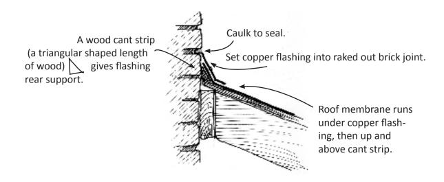
Copper flashing and roof membrane are not adhered to each other so they can move independently as adjacent structures move at different rates.
