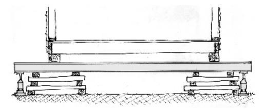
As building is lifted, add cribbing beams as soon as a new row will fit. When building is supported by cribbing beams, remove brick piers.
