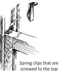
screwed to the top of sash. Spring clips that are screwed to the jamb.
