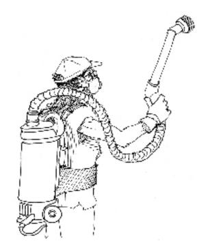
2. Once dry, vacuum all surfaces including electric outlet boxes and open ducts using a HEPA or high efficiency vacuum cleaner. A back-pac vacuum (for example, Pro-Team) is ideal for working off ladders, cleaning floors and crevices, and doing integrated pest management (IPM) work.
