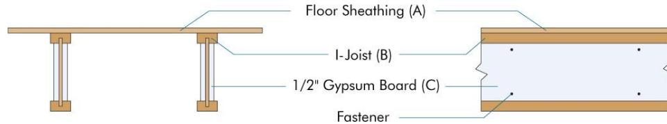
(A) **Floor Sheathing:** Materials and installation must be per 2015 IRC or 2012 IRC Section R503
