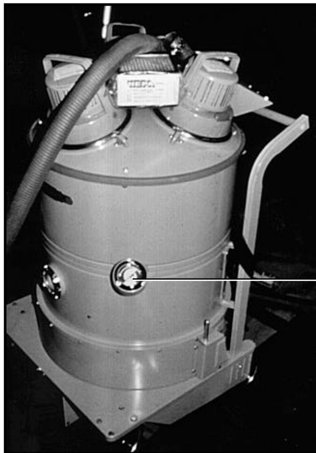
Figure 14.1b Pressure Gauge Indicator Shows When Filters Require Changing.
