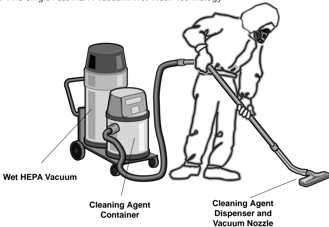
Figure 14.5 Single-Pass HEPA Vacuum/Wet Wash Technology.
