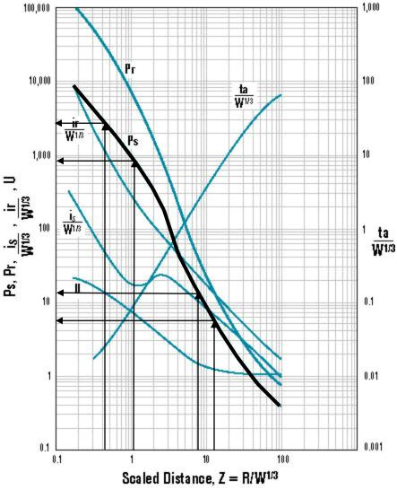
The peak positive incident pressures (Ps) are as follow: At 3 feet standoff distance: Z = 0.423, the Ps = 2,800 psi At 9 feet standoff distance: Z = 1.27, the Ps = 800 psi At 50 feet standoff distance: Z = 7.04, the Ps = 15 psi At 100 feet standoff distance: Z = 14.08, the Ps = 5.6 psi The substance being assessed (propane gas) poses the following hazards:
