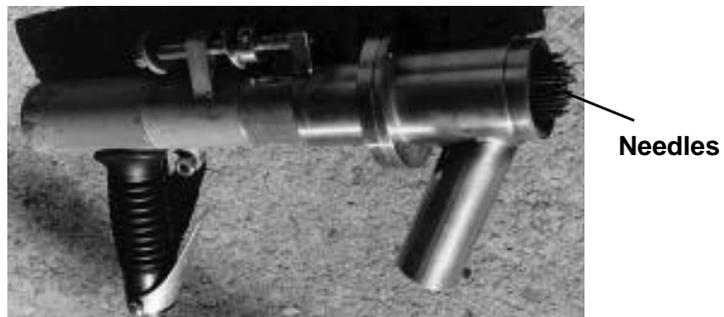
Figure 12.19a. Needle Gun With HEPA Exhaust Ventilation (without shroud).
